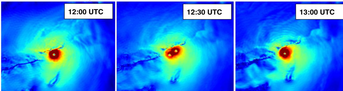
A similar artefact appears when performing weather nowcasting. This technique uses wind speed to advect thunderstorm cells. If the wind is very strong, it may result in discontinuous patches of thunderstorm cells without overlaps.
