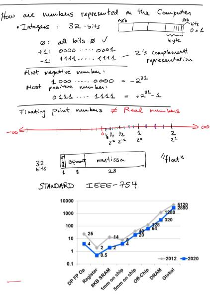
Figure 5: Energy cost, in picojoules (pJ) per 64-bit floating-point operation, for various common operations within a computer. The upper (gray) line characterizes energy cost estimates in 2012 technology, and the lower (blue) line projects costs in 2020. Note that the double-precision floating-point arithmetic (DP FP Op) energy cost is comparable to that for moving the same data 1mm-5mm on chip; that cost is dwarfed by the cost of any movement of this same data off chip.
